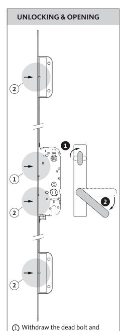
knob with a single 90° turn. (2) Press down the lever to withdraw the locking points and open the door.
