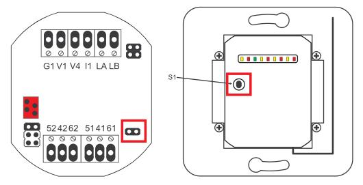
The housing cover must be opened to do this. Disconnect the module from the bus. Insert the jumper next to the terminal "51 41 61". Now press push-button "S1" until an acoustic signal is heard. The pairing information has been deleted.
