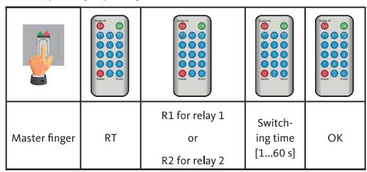
Fingerprint scanner and code keypad
