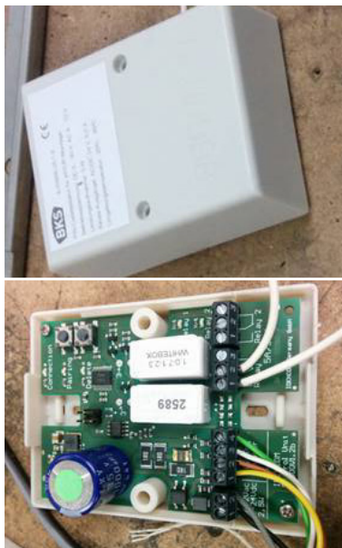
White box (relay unit)
