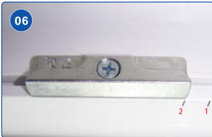
OPEN SASH ON TABLE TO INSTALL KEEPERS AROUND FRAME AND FASTEN WITH TYPE "D1" SCREWS (ALIGN EDGE OF KEEPER AS SHOWN)
