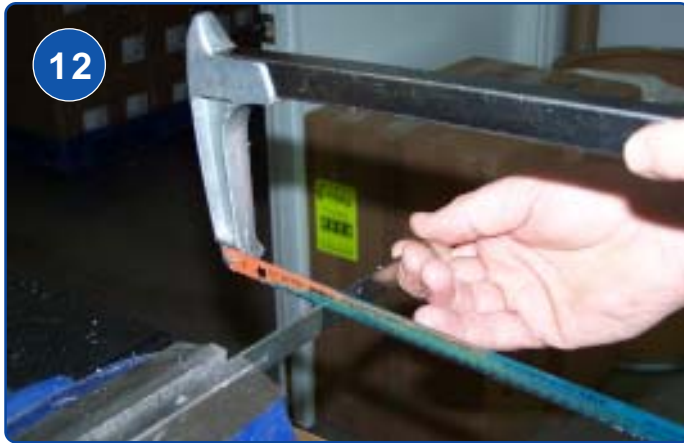
12 BEFORE CUTTING, FACE PLATE & DRIVING ROD MUST BE FLUSH AT BOTH ENDS
