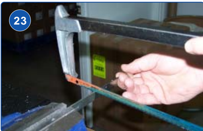
23 BEFORE CUTTING, FACE PLATE & DRIVING ROD MUST BE FLUSH AT BOTH ENDS
