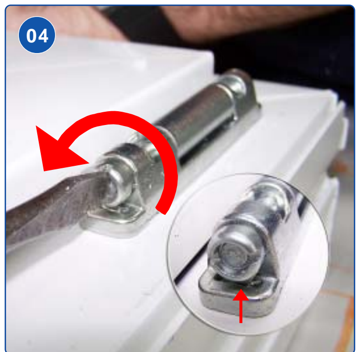
USE FLAT SCREW DRIVER TO TURN PIN 90° COUNTER CLOCKWISE TO LOCK OUT POSITION
